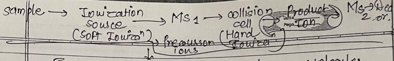
Ions collid = background gas molecules broken into smaller ions
